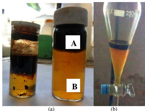
**Figure 2.** (a) Pyrolysis condensate separating into two distinct layers: portion labelled A is the viscous phase and B is the aqueous phase. (b) Separation of the phases using a separating funnel.
