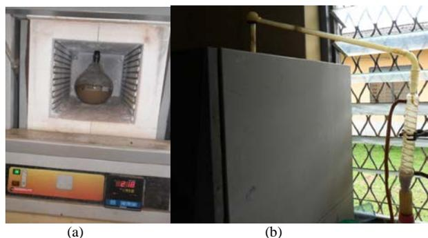
**Figure 1.** Modified slow pyrolysis set up showing (a) pyrex glass reactor in the muffle furnace (b) glass tubes conveying product gas to the reflux condenser.
