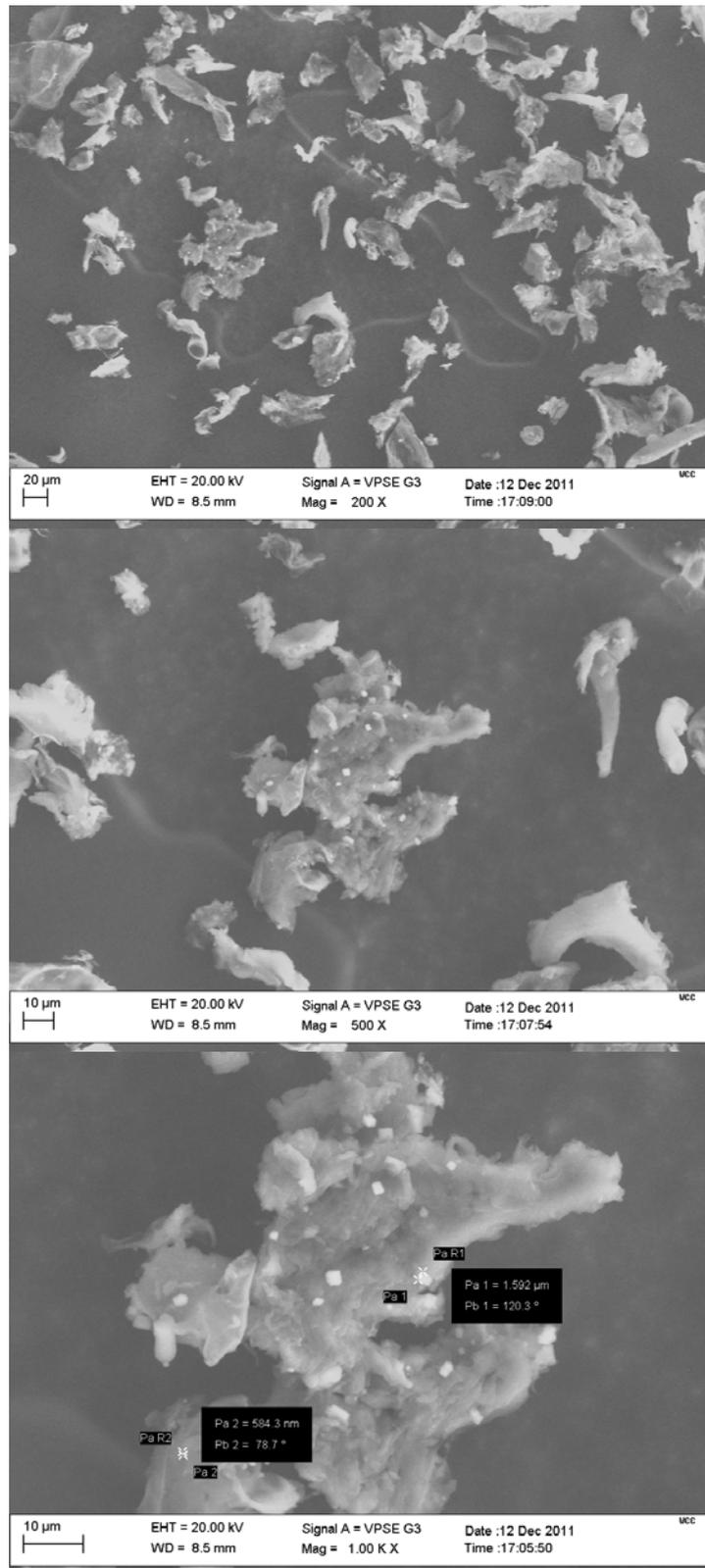
**Figure 5.** Scanning electron micrographs of bio-char of White corn cob at 200X, 500X and 1000X.
