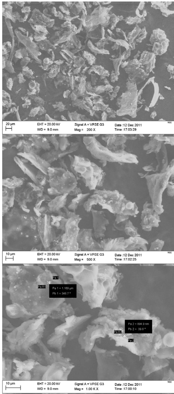
**Figure 4.** Scanning electron micrographs of bio-char of Yellow corn cob at 200X, 500X and 1000X.
